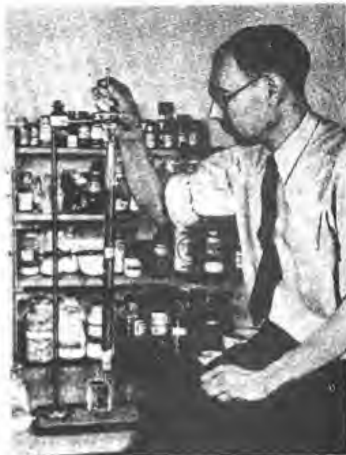
To prove that soil readily absorbs potassium, let a solution of potassium chloride or potassium carbonate seep through soil in this apparatus. The liquid that comes out contains hardly any of the potassium
